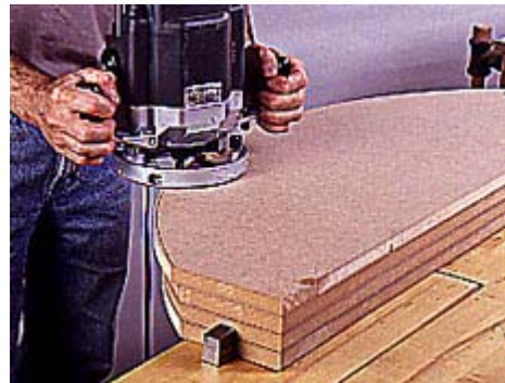
1 Make the bending form template with a plunge router on a trammel arm. Cut an arc in a sheet of MDF.
