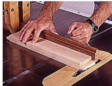
16 Clamp a stop to the mitre gauge fence. Use a dado blade to cut the tenons on the rails, stretchers and back slats.
