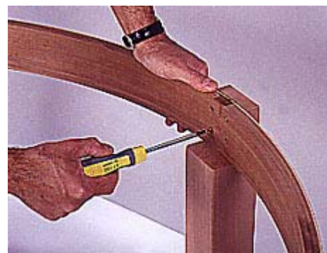
9 Glue and clamp together the half-lapped rail assembly. Check that the parts are square to one another.
