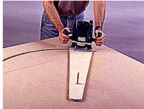
1 Make the bending form template with a plunge router on a trammel arm. Cut an arc in a sheet of MDF.
